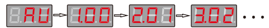
Initialize the assigned address AU CH1 Address is 00 CH2 Address is 01 CH3 Address is 02
